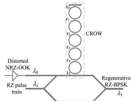
Fig. 1. Regenerative NRZ-OOK to RZ-BPSK format converter.
